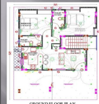
PROJECT NAME : ARAVIND RESIDENCE, BANGALORE. PLOT SIZE : 30 x 40, G+3. PLAN DETAILS : GROUND & TYPICAL FLOOR ELECTRICAL PLAN
